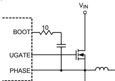
Figure 3. Reducing the UGATE Rise Time
