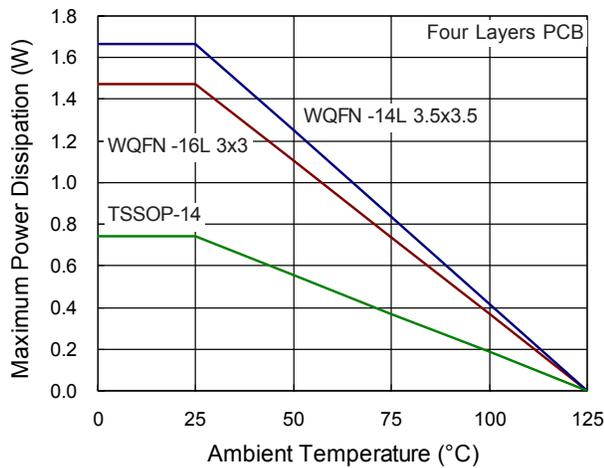
Figure 5. Derating Curves for RT8209A/B/C Packages
