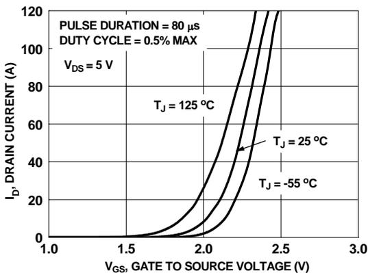
Figure 18. Transfer Characteristics
