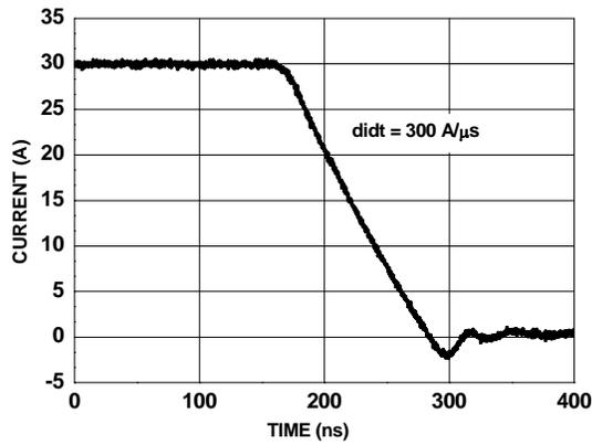
Figure 27. FDMS3660S SyncFET body diode reverse recovery characteristic
