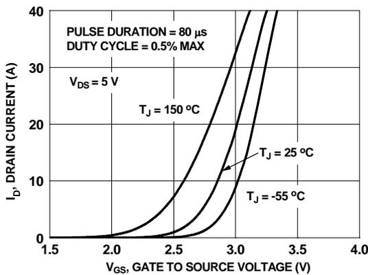
Figure 5. Transfer Characteristics
