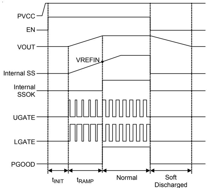
Figure 8. Internal Soft-Start Sequence
