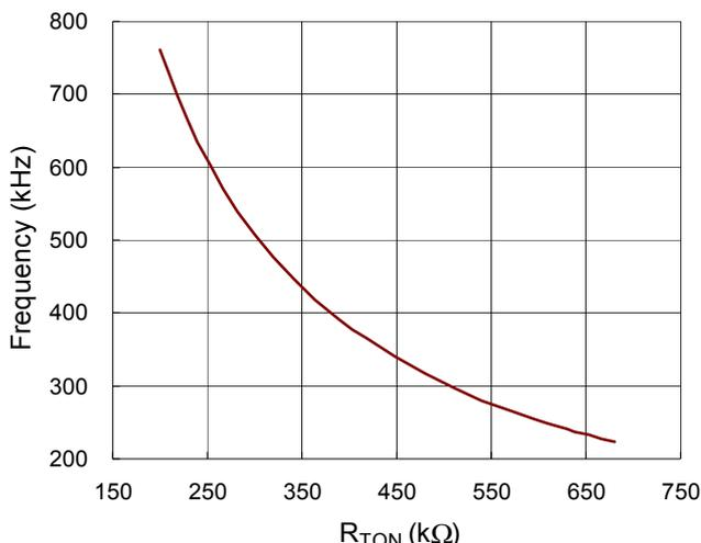
Figure 6. Frequency vs. R<sub>TON</sub>
