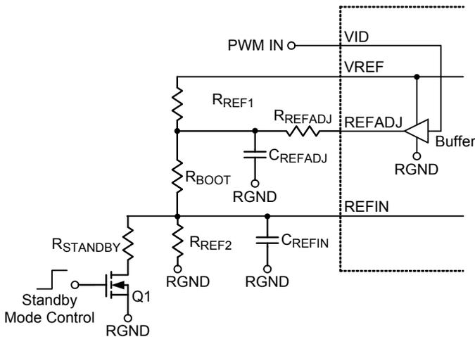
Figure 9. PWM VID Analog Circuit Diagram
