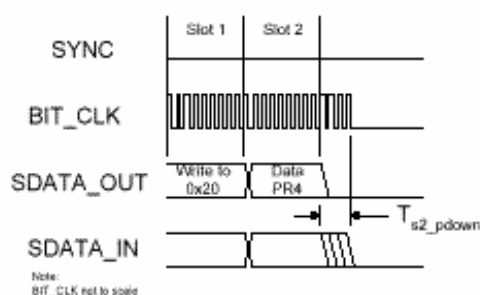
AC-Link low power mode timing diagram
