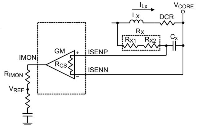
Figure 10. Lossless Current Sense Method for Single Phase
