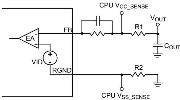
Figure 19. Remote Sensing Circuit
