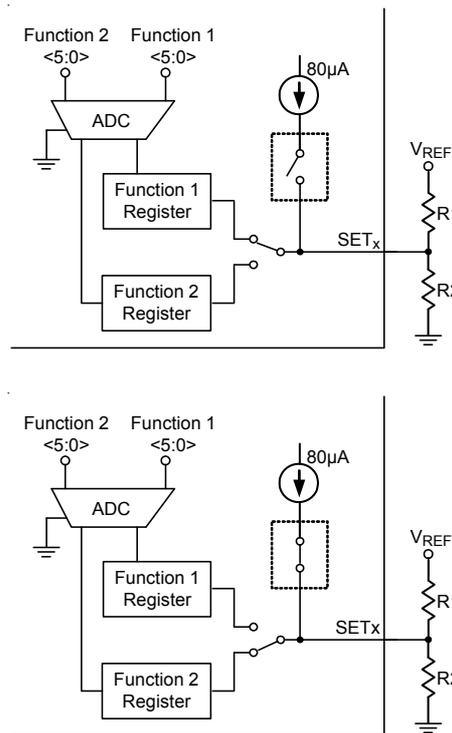
Figure 4. Multi-Function Pin Setting Mechanism for SET [1:3]
