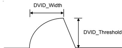
Figure 22. Definition of Virtual Charge Current Signal
