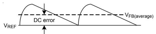
Figure 1. Average Output Voltage Control Loop Operation
