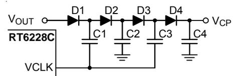
Figure 3. Charge Pump Circuit Connected to VCLK
