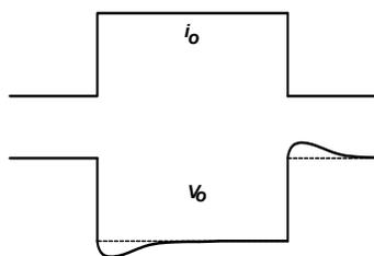
FIGURE 17. LOAD TRANSIENT RESPONSE WHEN  $C_n$  IS TOO SMALL
