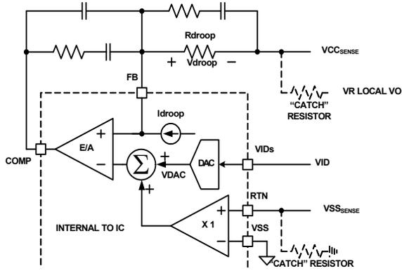
**FIGURE 8. DIFFERENTIAL SENSING AND LOAD LINE IMPLEMENTATION**
