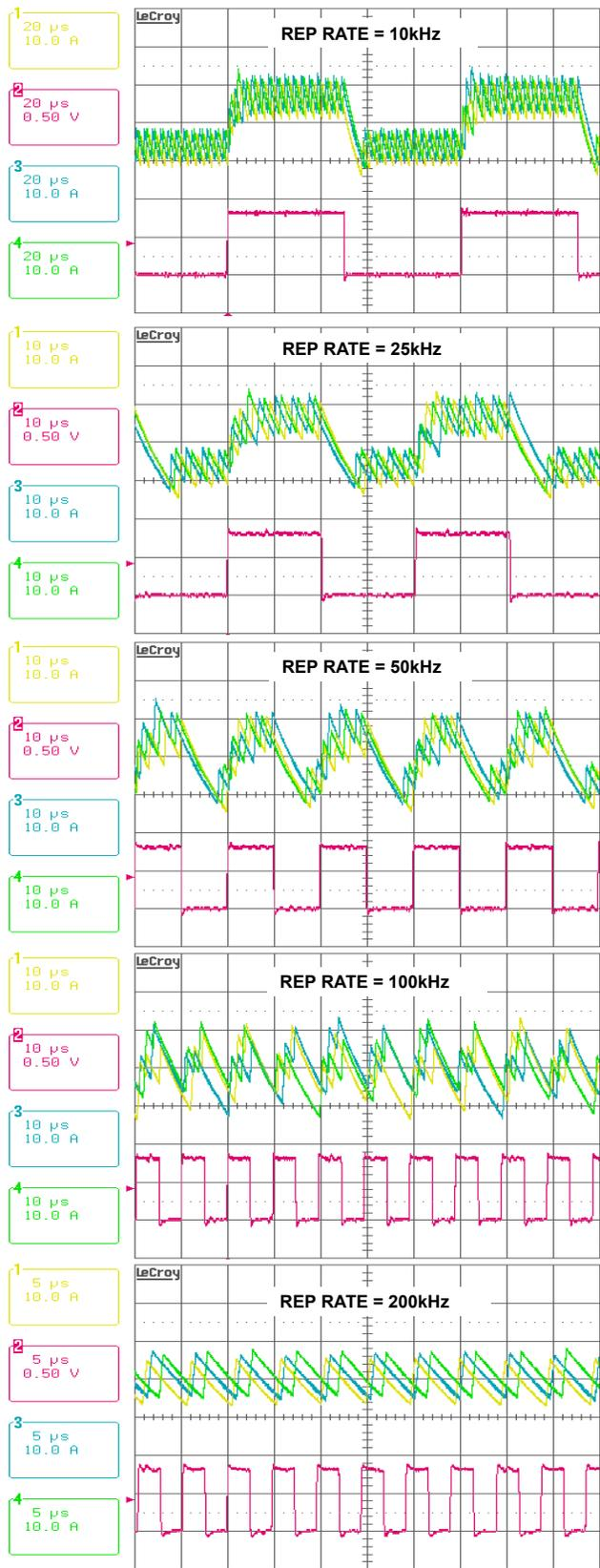
**FIGURE 11. CURRENT BALANCING DURING DYNAMIC OPERATION. CH1: IL1, CH2: I<sub>LOAD</sub>, CH3: IL2, CH4: IL3**
