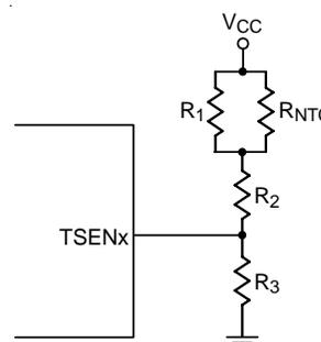
Figure 13. Thermal Monitoring Circuit
