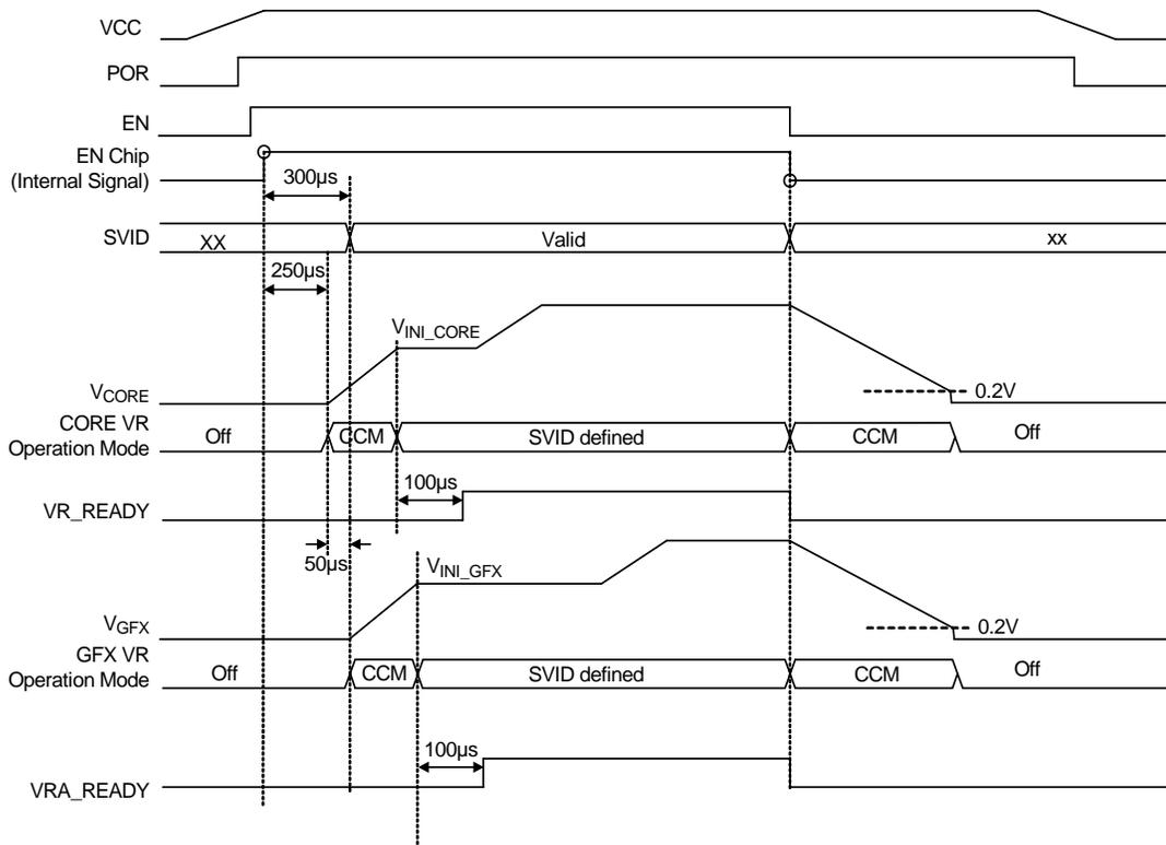
Figure 7 (b). Power sequence for RT8167B ( $V_{INI\_CORE} \neq 0$ ,  $V_{INI\_GFX} \neq 0V$ )
