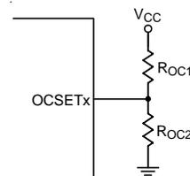
Figure 14. OCP Setting without Temperature Compensation
