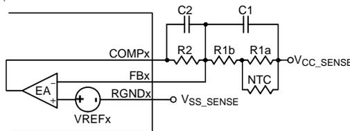
Figure 10. Loop Setting with Temperature Compensation
