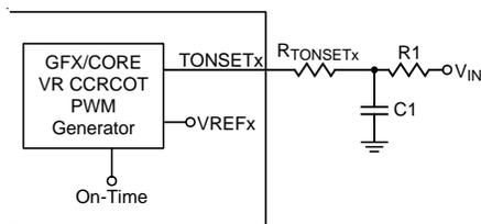
Figure 11. On-Time Setting with RC Filter
