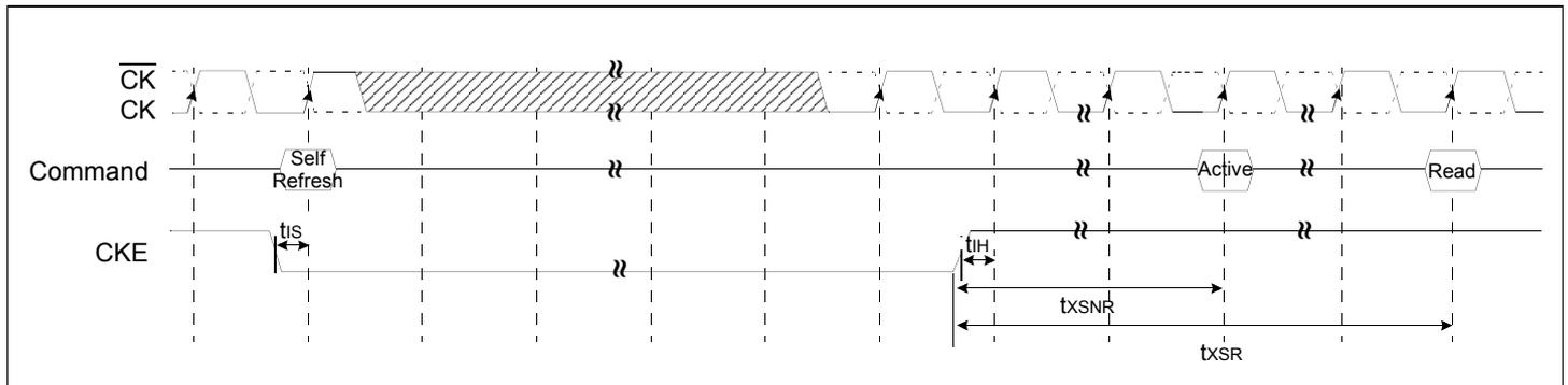
\* Once the device enters the power down mode, it should be in NOP state at least for 10ns. The minimum duration for the power down mode once CKE brought to down should be at least 10ns.
