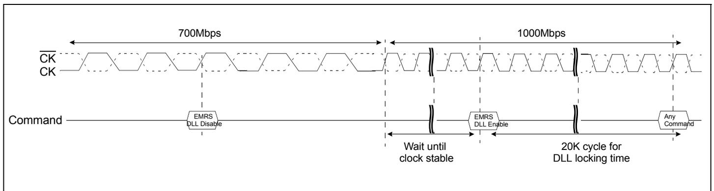
**Figure 1. Clock frequency change sequence after the power-up(example)**
