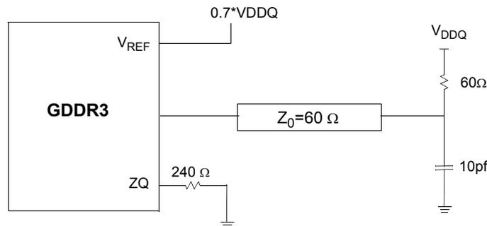
**NOTE :** 1. Outputs measured into equivalent load of 10pf at a driver impedance of 40 Ω.
