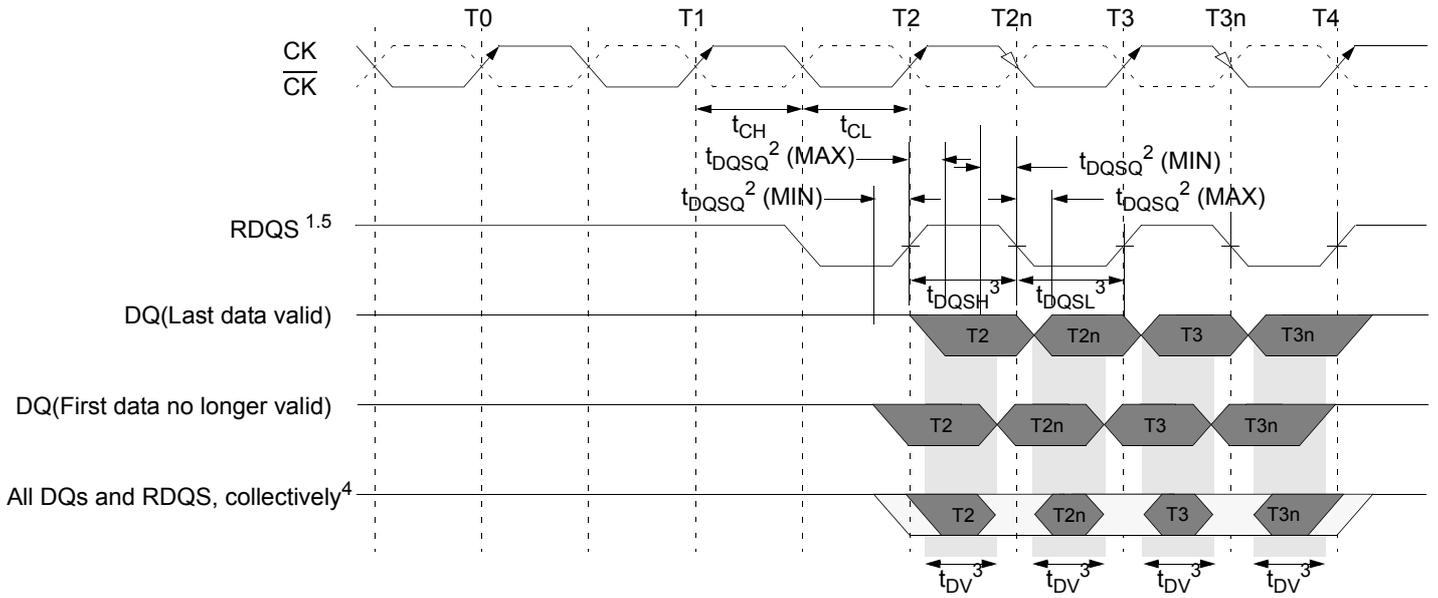
Figure 9. Data Output Timing (1) -  $t_{DQSQ}$ ,  $t_{QH}$  and Data Valid Window
