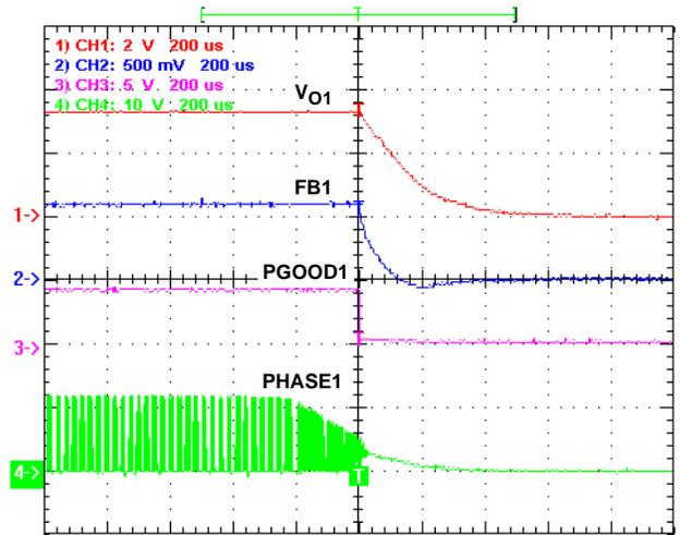
FIGURE 8. POWER-OFF,  $V_{IN} = 12V$ ,  $I_O = 5A$ ,  $V_O = 3.3V$
