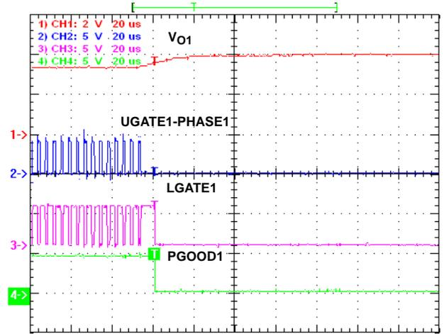
FIGURE 22. TRI-STATE OVERVOLTAGE PROTECTION,
