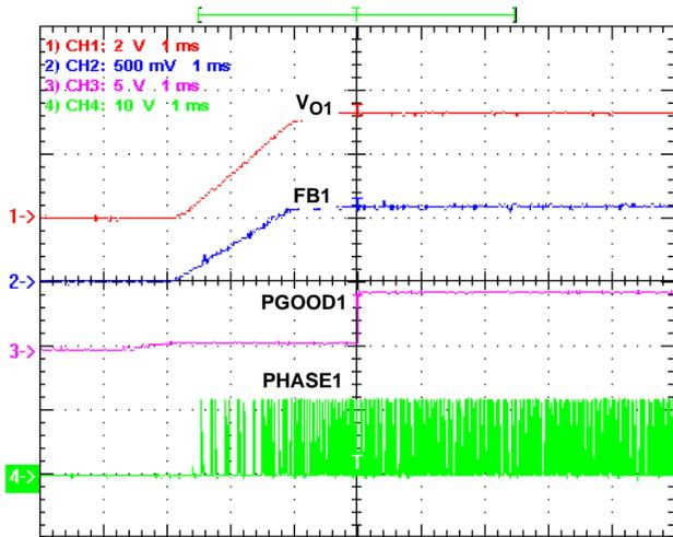
FIGURE 7. POWER-ON,  $V_{IN} = 12V$ ,  $I_O = 5A$ ,  $V_O = 3.3V$
