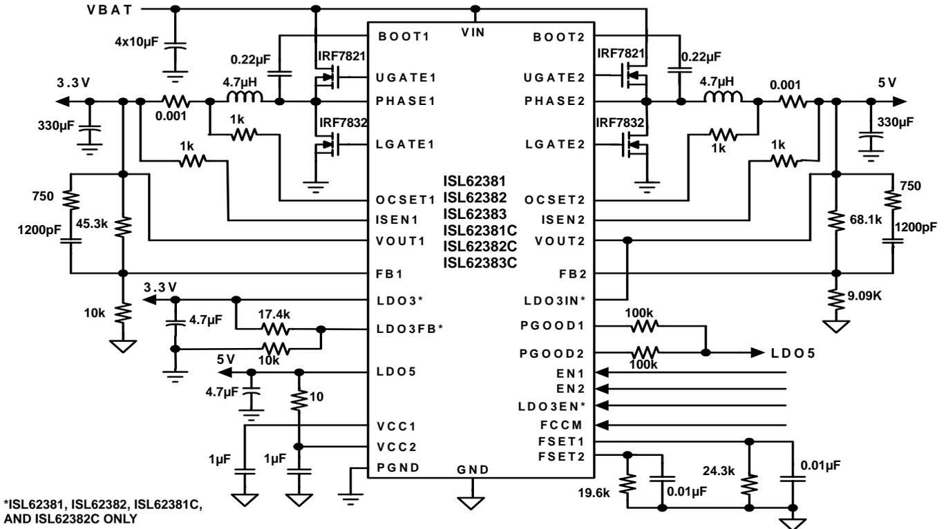
FIGURE 2. TYPICAL APPLICATION CIRCUIT WITH RESISTOR CURRENT SENSE
