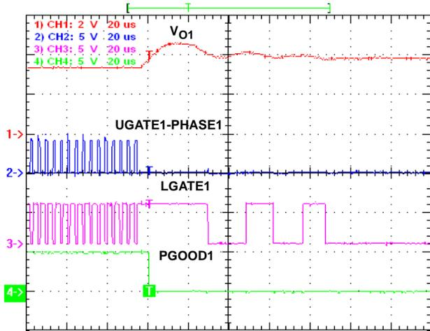
FIGURE 21. CROWBAR OVERVOLTAGE PROTECTION,
