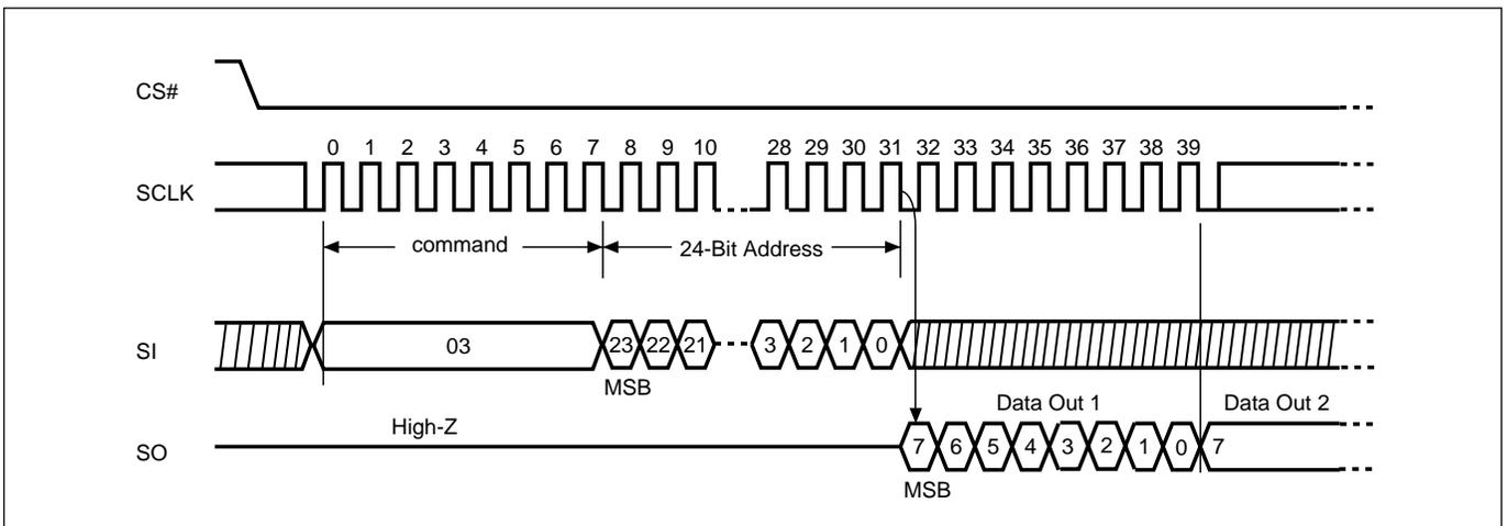
**Figure 17. Read at Higher Speed (FAST\_READ) Sequence (Command 0B)**
