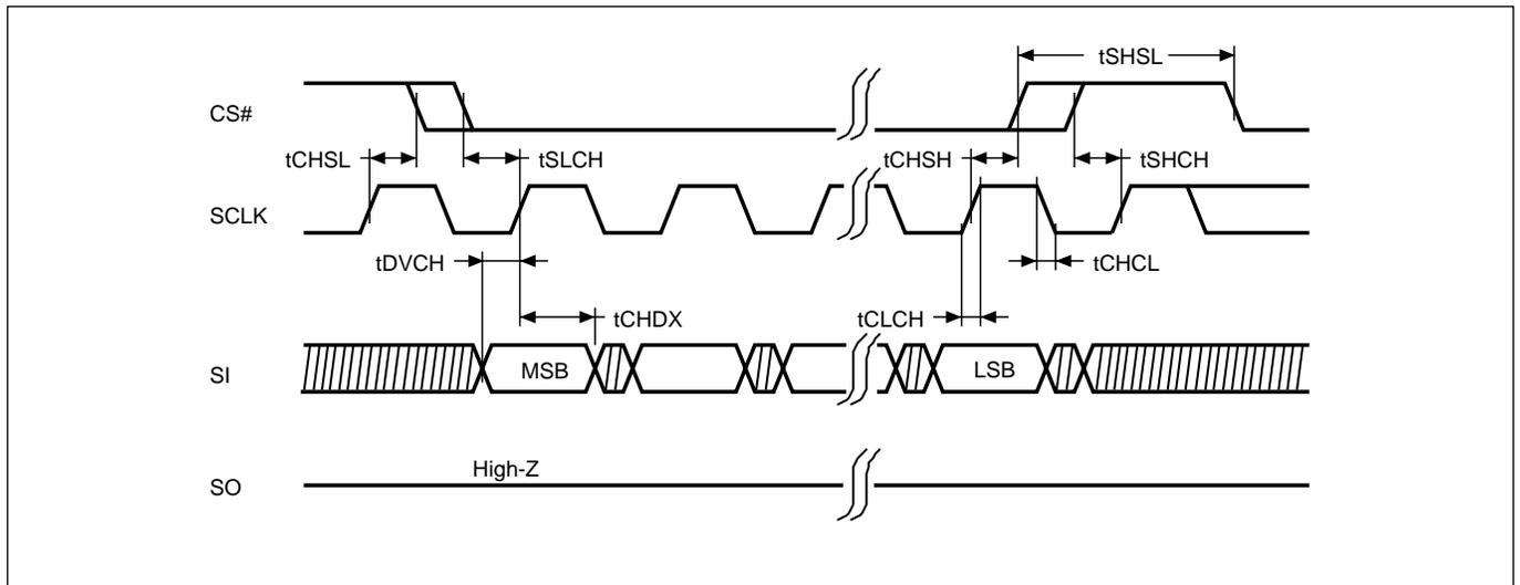
**Figure 8. Output Timing**
