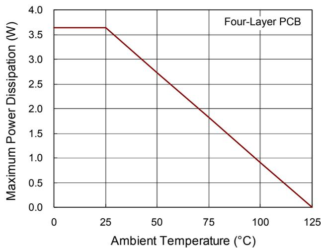
Figure 17. Derating Curve of Maximum Power Dissipation
