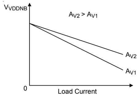
Figure 14. VDDNB Controller : Error Amplifier gain (Av) Influence on V<sub>VDDNB</sub> Accuracy
