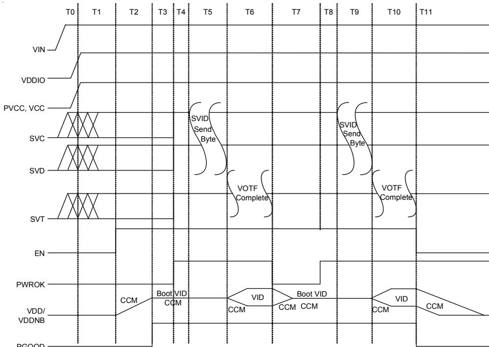
Figure 2. Simplified Sequence Timing Diagram
