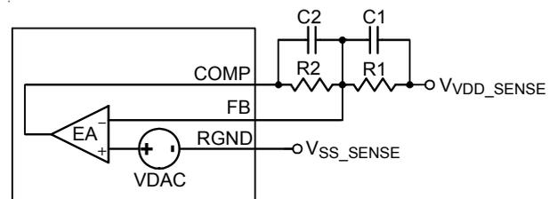
Figure 9. VDD Controller: Compensation Circuit
