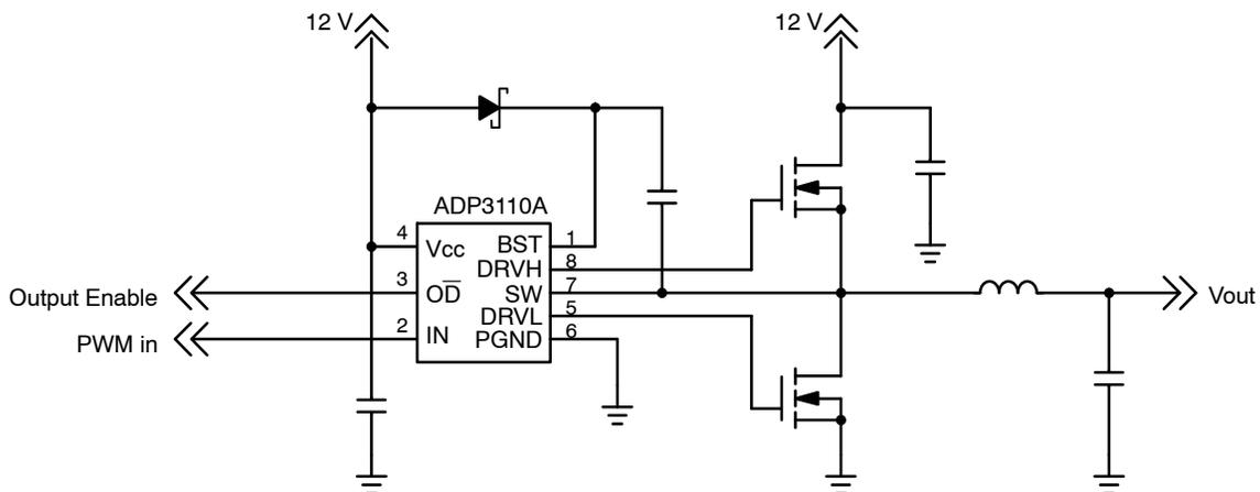
Figure 4. ADP3110A Example Circuit
