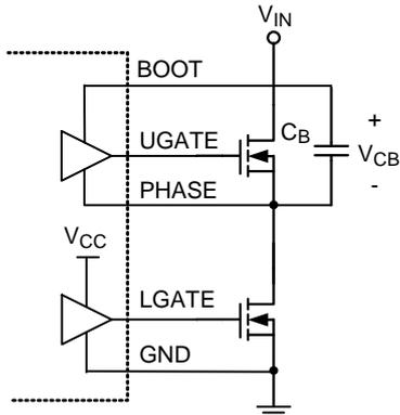
Figure 2. Part of Bootstrap Circuit of RT9611C/D
