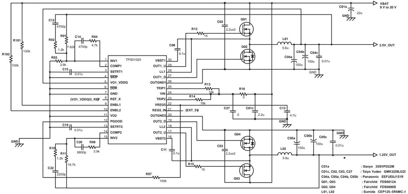
Figure 6. Typical Application Circuit: DDR(2.5V/6A + 1.25V/6A) from VBAT
