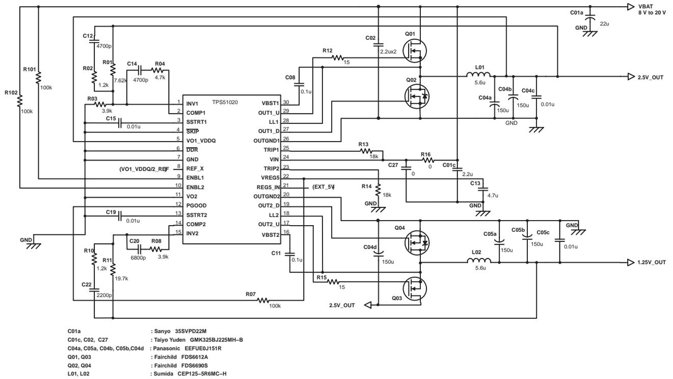
Figure 7. Typical Application Circuit: DDR (2.5V/6A + 1.25V/3A) Cascade
