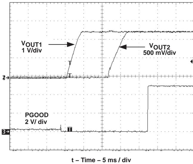
Figure 18. Simultaneous Startup
