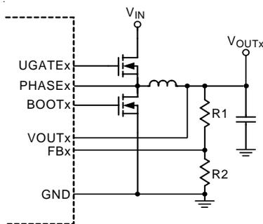
Figure 6. Setting VOUTx with a Resistor-Divider
