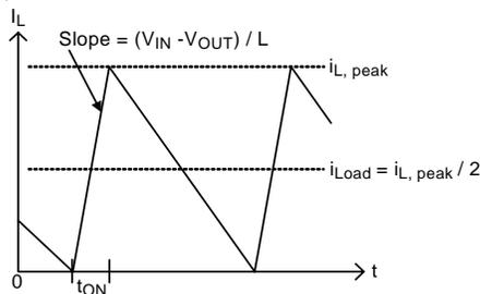
Figure 3. Boundary Condition of CCM/DCM
