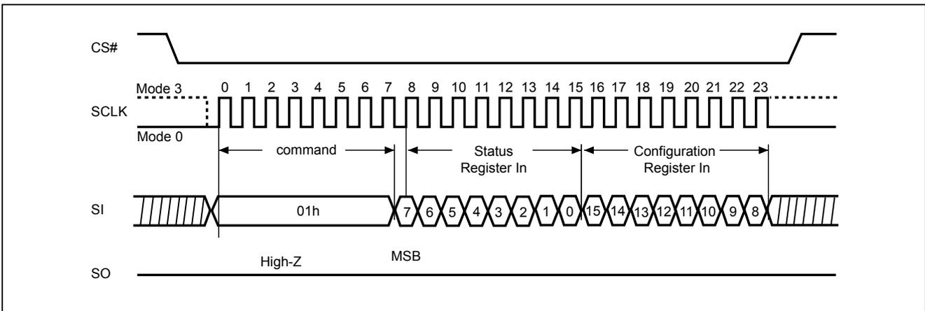
The CS# must go high exactly at the byte boundary; otherwise, the instruction will be rejected and not executed. The self-timed Write Status Register cycle time (tW) is initiated as soon as Chip Select (CS#) goes high. The Write in Progress (WIP) bit still can be checked out during the Write Status Register cycle is in progress. The WIP sets 1 during the tW timing, and sets 0 when Write Status Register Cycle is completed, and the Write Enable Latch (WEL) bit is reset.
