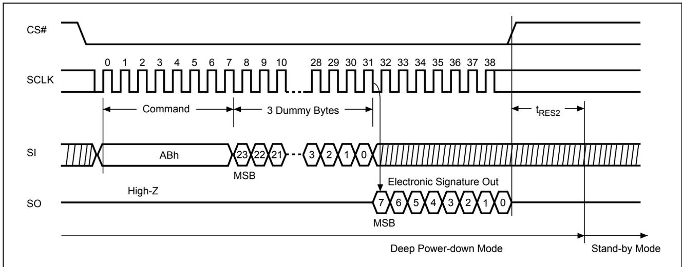
**Figure 26. Release from Deep Power-down (RDP) Sequence**
