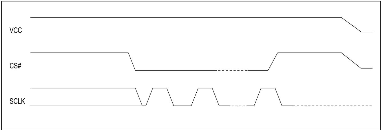
**Figure 44. Power-up Timing**
