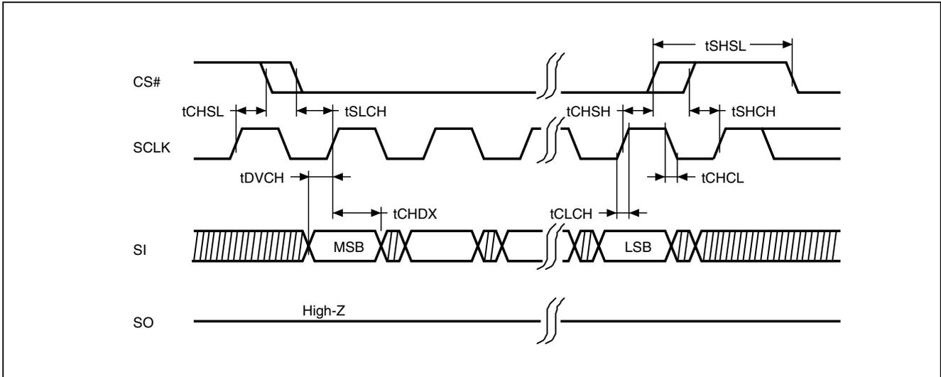
**Figure 41. Output Timing**
