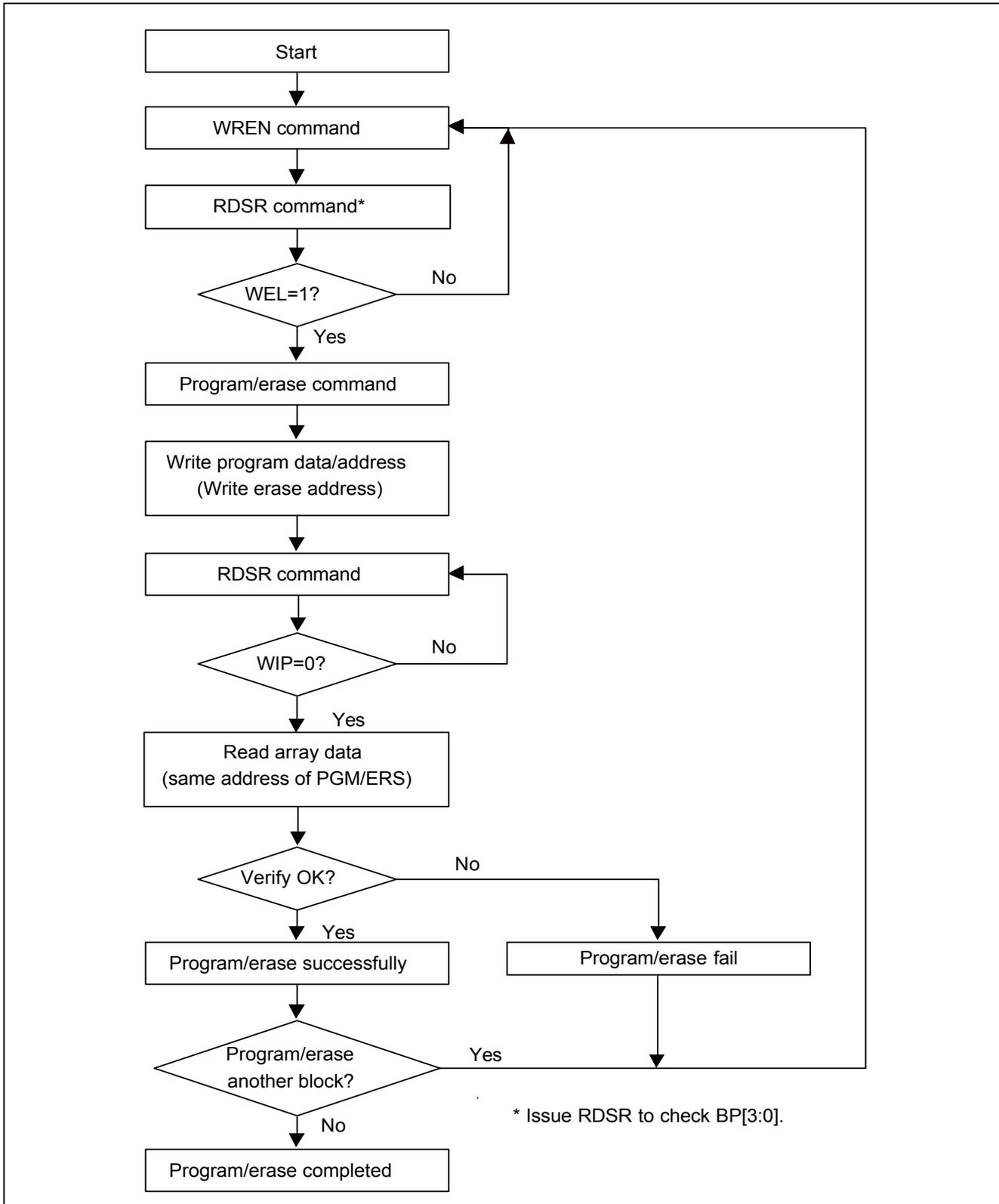
**Figure 23. Program/Erase Flow(2) without read array data**
