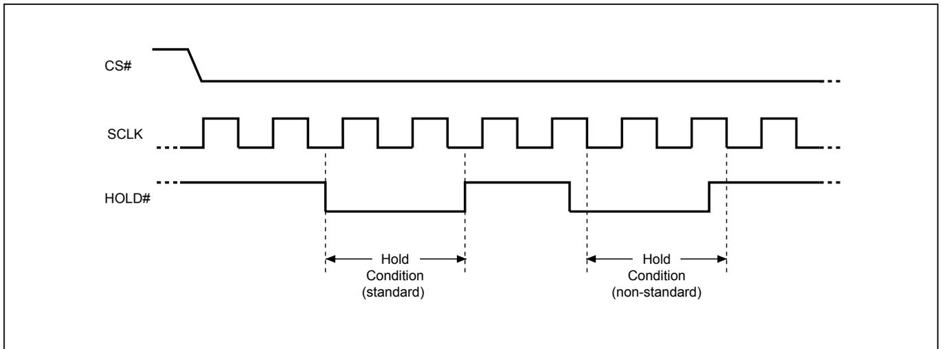
The Serial Data Output (SO) is high impedance, both Serial Data Input (SI) and Serial Clock (SCLK) are don't care during the HOLD operation. If Chip Select (CS#) drives high during HOLD operation, it will reset the internal logic of the device. To re-start communication with chip, the HOLD# must be at high and CS# must be at low.
