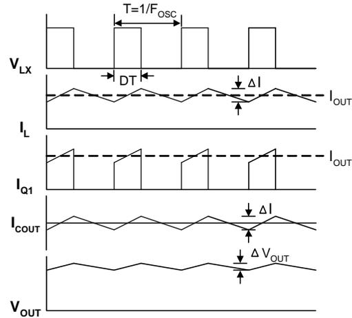
Figure 1. Converter Waveforms
