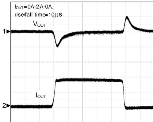
CH1:  $V_{OUT}$ , 200mV/Div, offset=3.3V
