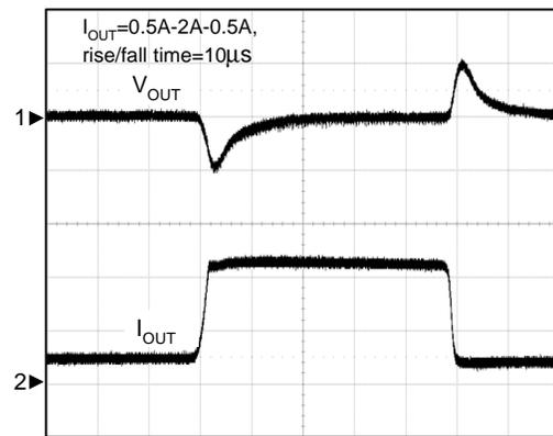
CH1:  $V_{OUT}$ , 200mV/Div, offset=3.3V
