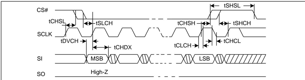
**Figure 43. Output Timing**
