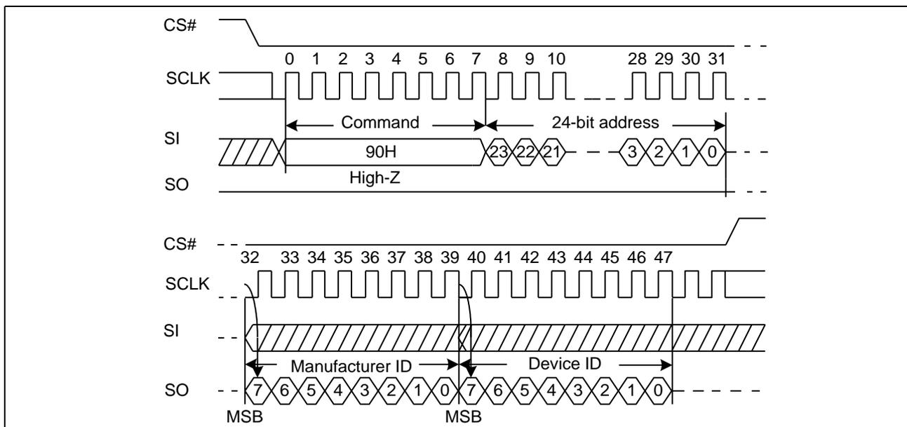
**7.24. Dual I/O Read Manufacture ID/ Device ID (92H)**
