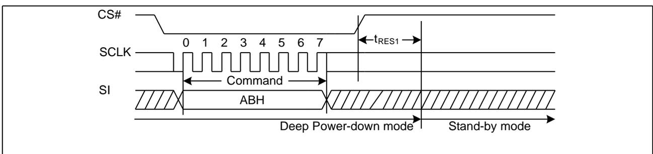
Figure 26. Release Power-Down/Read Device ID Sequence Diagram
