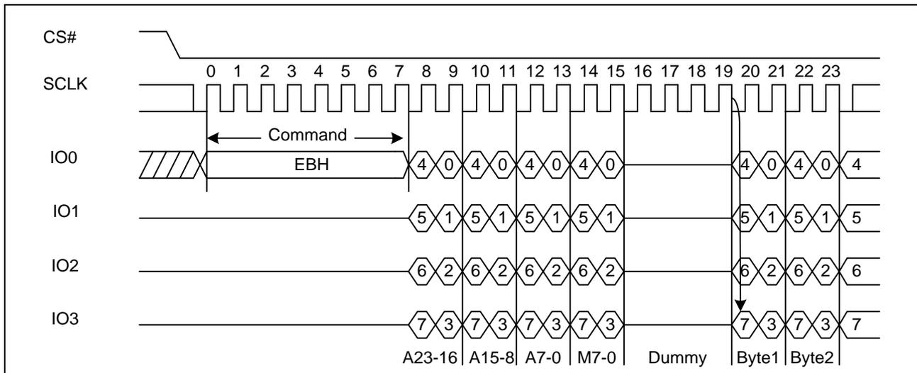
**Figure 13. Quad I/O Fast Read Sequence Diagram (M5-4= (1, 0))**
