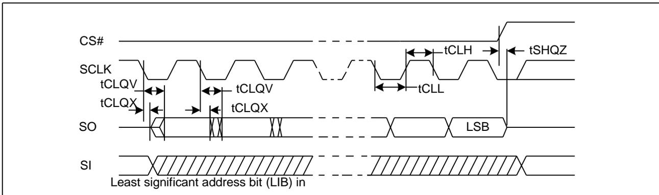
**Figure 44. Resume to Suspend Timing**
