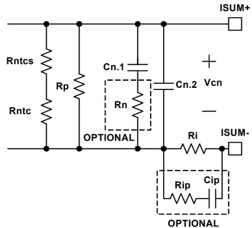
FIGURE 22. OPTIONAL CIRCUITS FOR RING BACK REDUCTION
