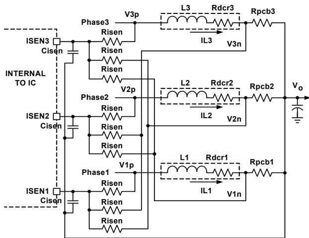
**FIGURE 12. DIFFERENTIAL-SENSING CURRENT BALANCING CIRCUIT**
