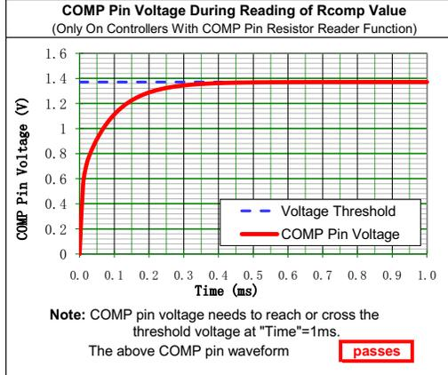
FIGURE 27. SCREENSHOT OF THE COMPENSATOR DESIGN SPREADSHEET
