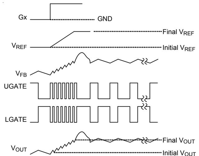
Figure 4. Output Voltage Up Transition with Overshooting
