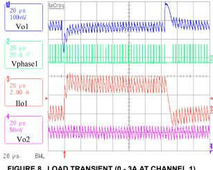
FIGURE 8. LOAD TRANSIENT (0 - 3A AT CHANNEL 1) (FORCED PWM MODE)
