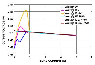
FIGURE 3. OUTPUT VOLTAGE OF CHANNEL 1 vs LOAD
