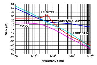
FIGURE 39. THE BODE PLOT OF THE LC FILTER,
