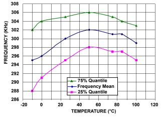
FIGURE 5. SWITCHING FREQUENCY OVER TEMPERATURE
