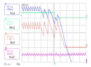
FIGURE 19. OVERCURRENT PROTECTION AT CHANNEL 1
