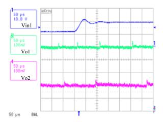
FIGURE 12. INPUT STEP-UP TRANSIENT AT HYS MODE
