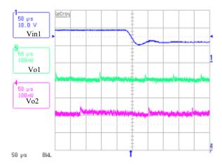
FIGURE 14. INPUT STEP-DOWN TRANSIENT AT HYS MODE
