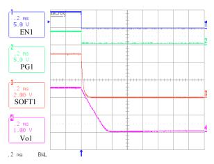
FIGURE 23. SOFT SHUTDOWN INTERVAL
