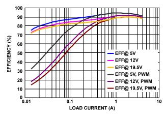
FIGURE 2. EFFICIENCY OF CHANNEL 2, 1.8V, HYS/PWM MODE
