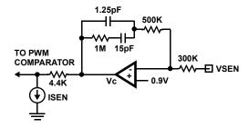
FIGURE 38. THE INTERNAL COMPENSATOR
