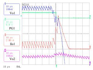
FIGURE 20. SHORT-CIRCUIT PROTECTION AT CHANNEL 1
