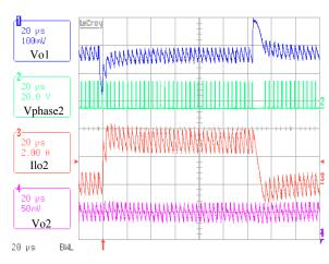
FIGURE 10. LOAD TRANSIENT (0 - 3A AT CHANNEL 2) (FORCED PWM MODE)
