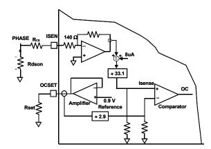
FIGURE 42. EQUIVALENT CIRCUIT FOR OC SIGNAL GENERATOR
