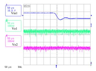
FIGURE 13. INPUT STEP-DOWN TRANSIENT AT PWM MODE
