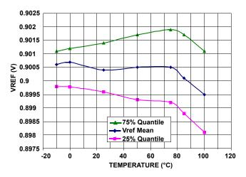
FIGURE 6. REFERENCE VOLTAGE ACCURACY OVER TEMPERATURE
