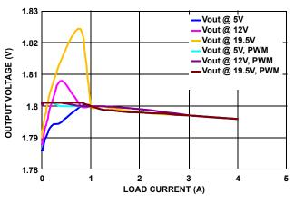
FIGURE 4. OUTPUT VOLTAGE OF CHANNEL 2 vs LOAD
