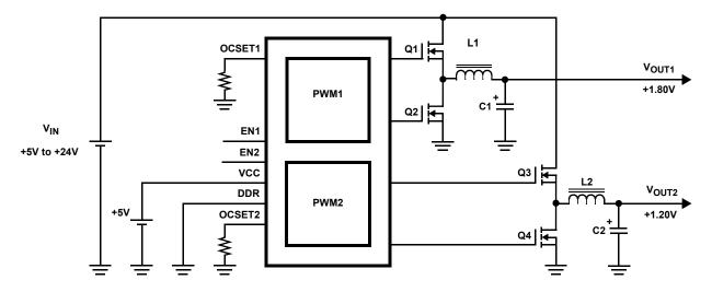
ISL6227 APPLICATION CIRCUIT FOR TWO CHANNEL POWER SUPPLY
