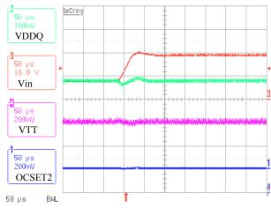
FIGURE 29. INPUT LINE TRANSIENT IN DDR MODE
