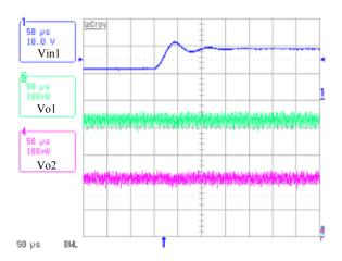
FIGURE 11. INPUT STEP-UP TRANSIENT AT PWM MODE
