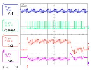
FIGURE 9. LOAD TRANSIENT (0 - 2A AT CHANNEL 2) (DIODE EMULATION MODE)
