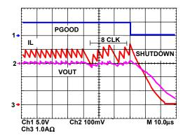
FIGURE 40. OVERCURRENT PROTECTION
