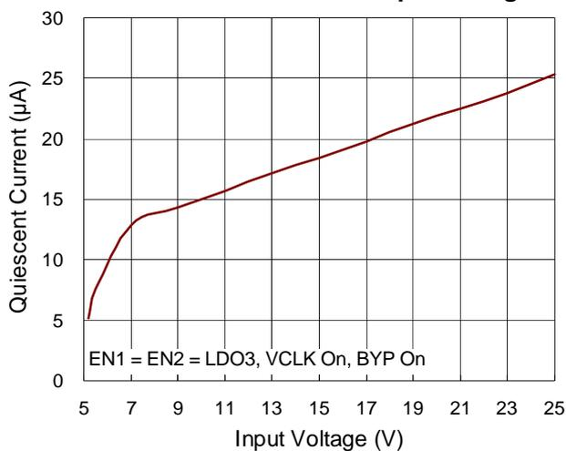
BYP1 Supply Current vs. Input Voltage
