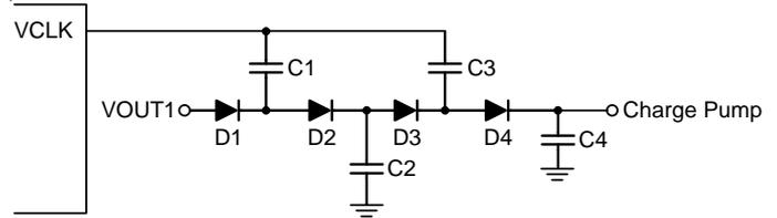
Figure 3. Charge Pump Circuit Connected to VCLK
