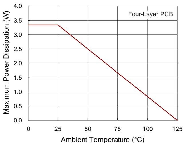
Figure 8. Derating Curve of Maximum Power Dissipation
