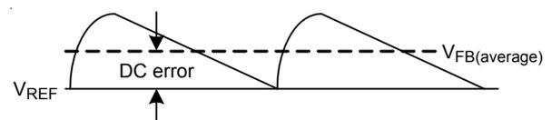
Figure 1. Average Output Voltage Control Loop Operation
