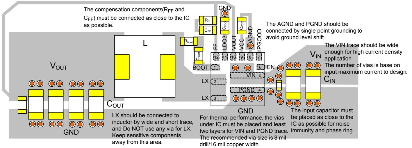
Figure 8. Layout Guide of RT6258B
