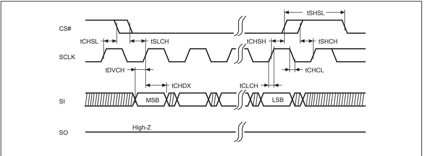
**Figure 8. Output Timing**
