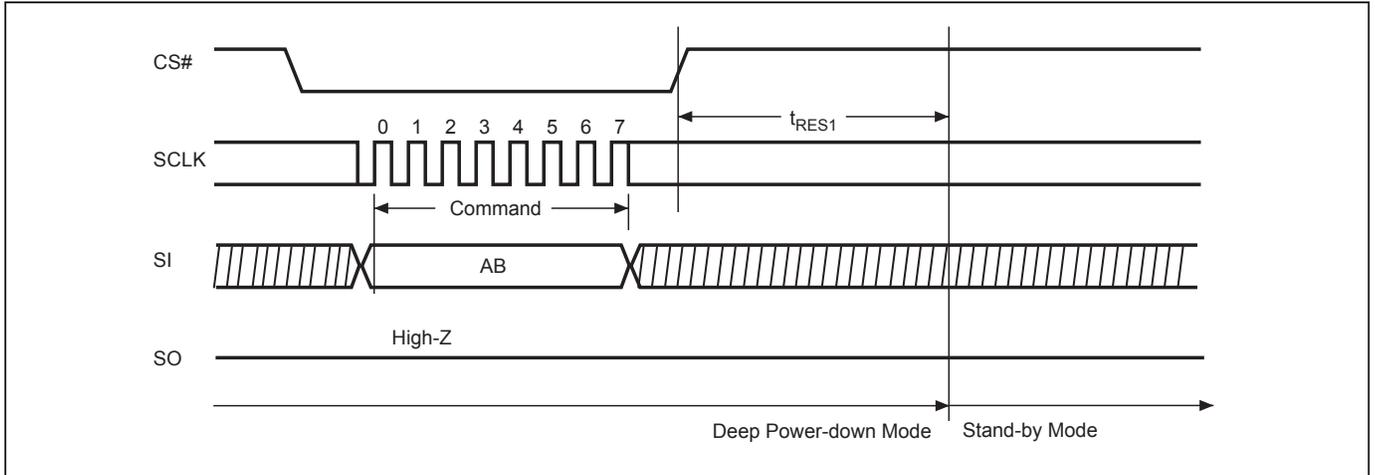
**Figure 25. Read Electronic Manufacturer & Device ID (REMS) Sequence (Command 90)**
