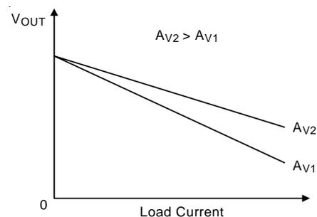
Figure 5. Error Amplifier Gain ( $A_v$ ) Influence on  $V_{OUT}$
