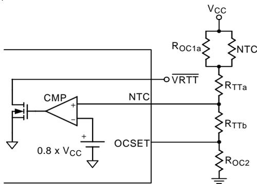
Figure 13. Using Single NTC Thermistor for Thermal Throttling and Current Limit Setting
